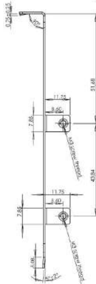
Figure 83: Dimensions Front Panel CIFX 50-CC or CIFX 50E-CC
